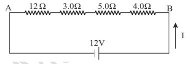
129 The equivalent resistance between points A and B, is
