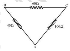
The resistance of side AB is 40 ohms, of side BC60 ohms and of side CA 100 ohms. The effective resistance between the point A and B in ohms is
