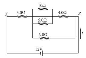
132 The equivalent resistance between points A and B
