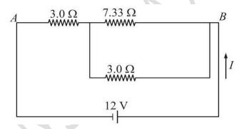
(ii) The  $7.33\Omega$  and the  $3.0\Omega$  are in parallel.
