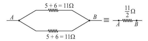
10 (a) To get the maximum resistance, all four resistors should be connected in series,
