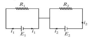
For any value of *E* or *R* current going from first loop to second loop must be zero.
