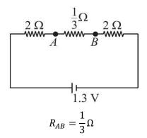
Then equivalent resistance across the battery,  $R_{eq}=2+\frac{1}{3}+2=\frac{13}{3}\Omega$
