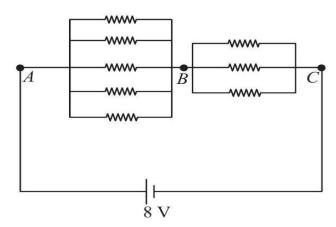
Resistance between arm AB,  $R_{\text{net }AB}=\frac{1}{5}k\Omega=\frac{1000}{5}\Omega$  Resistance between arm BC,  $R_{\text{net }BC}=\frac{1}{3}k\Omega=\frac{1000}{3}\Omega$
