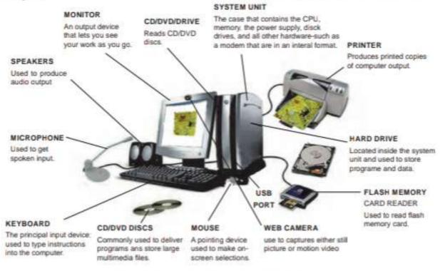
Fig: 1 Computer System and Peripherals
