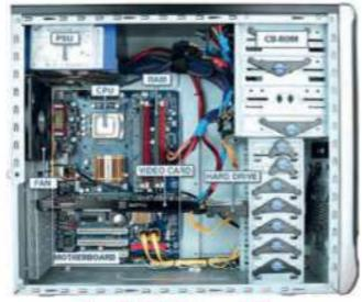
Fig: 3 CPU Internal View
