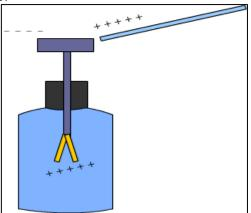
**Structure of Electroscope:** It is made of a glass jar. A vertical brass rod is inserted into the jar through a cork. The top of the brass rod has a horizontal brass rod or a brass disc. Two gold leaves are suspended from the brass rod; inside the jar.
