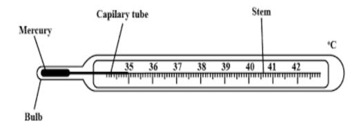
The stem, as well as bulb of laboratory thermometer, is longer when compared to the clinical thermometer. There is no kink in laboratory thermometer. It has only celsius scale. It can measure temperature from -10°C to 110°C.
