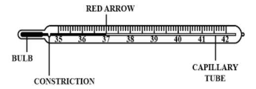
It can give temperature range from a minimum of 35°C or 94°F to the maximum of 42°C or 108°F. Fahrenheit scale is more sensitive than Celsius scale. Thus, the temperature is measured in Fahrenheit(°F).
