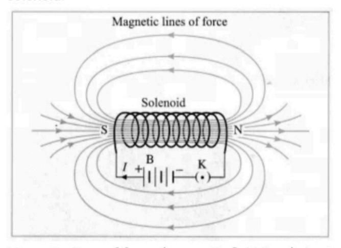
Magnetic lines of force (magnetic field lines) due to a current carrying solenoid.
