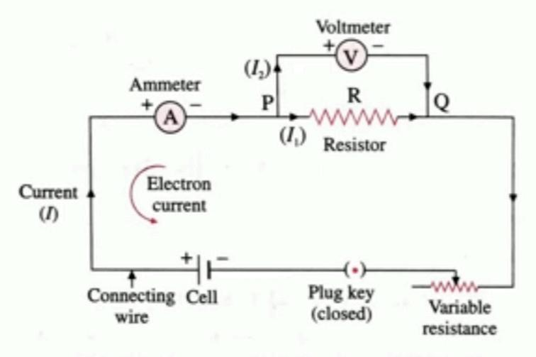
Circuit diagram showing how different components are connected.
