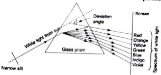
The white light consists of seven colours. The refractive Index of the medium also depends on the wavelength and speed of light. So, when white light enters into the glass prism, the prism material has a different refractive index for the different wavelengths. This causes the different colours to travel with the different velocities inside the glass prism in different directions.
