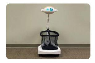
Budgee is a personal assistant robot designed by Five Elements Robotics to carry items for you. It follows a user-worn or carried ultrasonic transceiver and can carry up to 50 pounds. Budgee can be folded for easy storage and transportation, and it communicates with its user via a smartphone or tablet.
